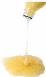
Distinguishing foam agents by their viscosity
